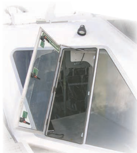
Side hung emergency exit
