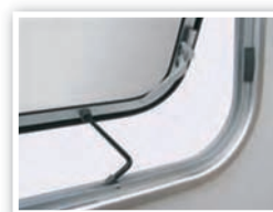
Deck hatch ventilation stay
